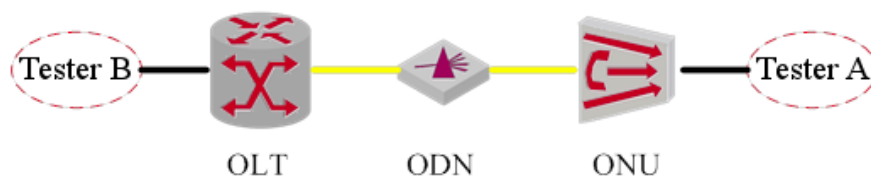
Configuration diagram for MAC authentication
