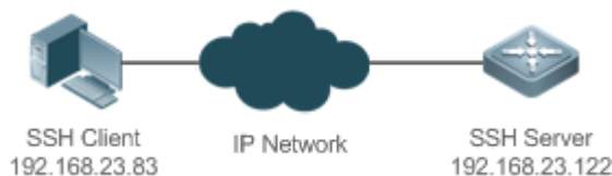
Figure 7-5 Networking Topology of SSH File Transfer
