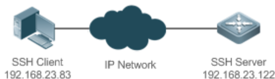
Figure 7-1 Networking Topology of SSH Device Management
