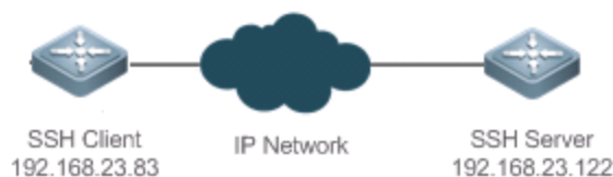
Figure 7-6 Networking Topology of SSH Client Application
