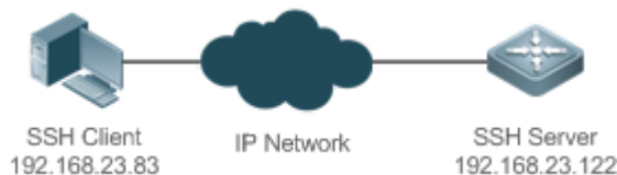
Figure 7-1 Networking Topology of SSH Device Management
