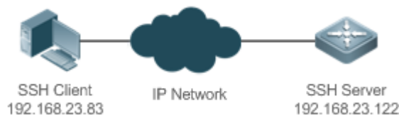
Figure 7-5 Networking Topology of SSH File Transfer
