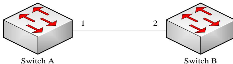
1. Configure the interface 1 that Switch A connects to Switch B to trunk:
