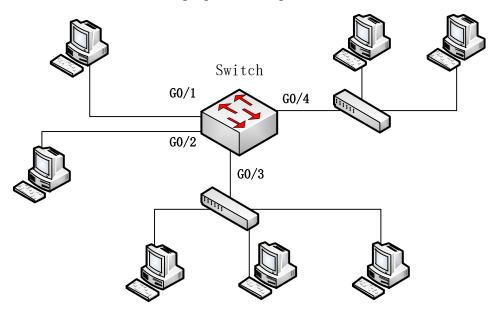
Sets the parameter of Filter. A host sending more than 100 ARP messages in 10s will be taken as an attack source.
