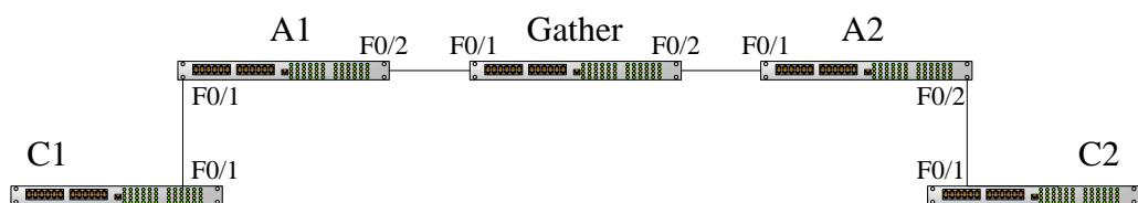
A1/A2/Gather belong to core network, C1/C2 are switches distributed in two places. Customer wants to combine two of its network to one , that is, the core network is a transparent transmission channel for the customer. If user wants to realize the transparent transmission of STP, then the following configurations should be configured on each switch:
