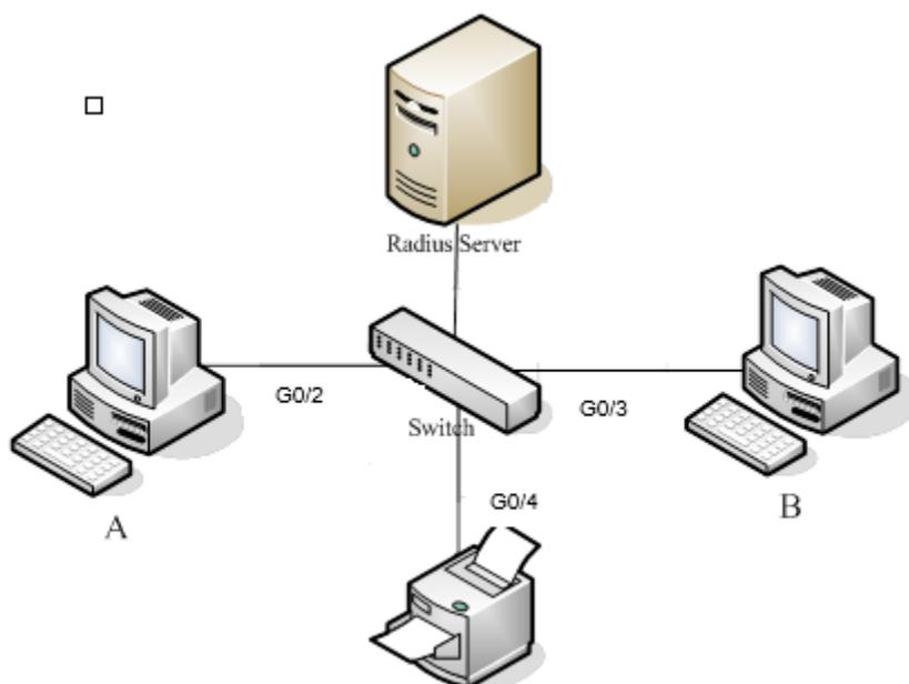
Host A connects the G0/2 interface of the OLT, host B the G0/3 interface, and host C the G0/4 interface; the radius-server host's IP is 192.168.20.2 and its key is TST; on the G0/2 interface the remote radius authentication, user-bind, accounting and re-authentication will be enabled altogether, on the G0/3 interface the local authentication, eap, multi-hosts and guest-vlan are enabled altogether, and on the
