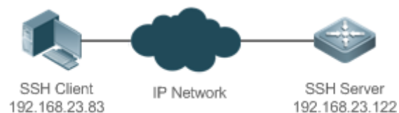
Figure 11-1 Networking Topology of SSH Device Management
