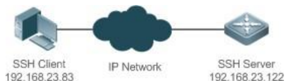
Figure 11-4 Networking Topology of SSH File Transfer
