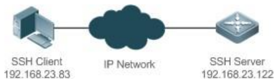
Figure 11-3 Network Topology for Public Key Authentication of SSH Users
