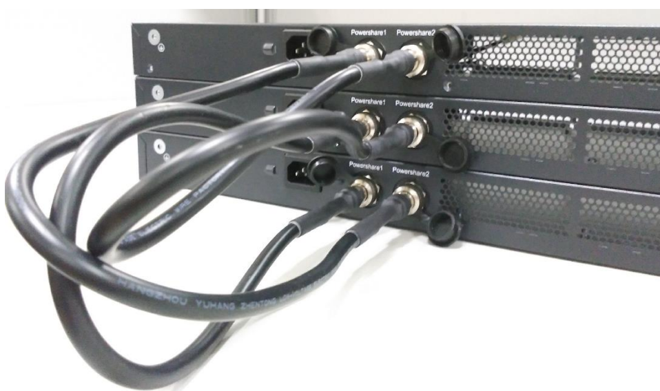
Figure 3-12 Connecting Cables Among Three Switches 3
