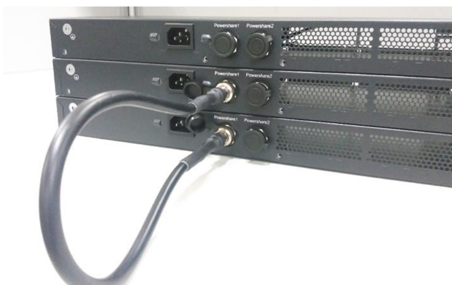
Figure 3-10 Connecting Cables among Three Switches 1
