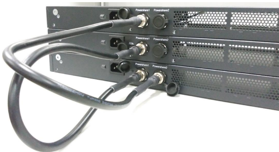
Figure 3-11 Connecting Cables Among Three Switches 2
