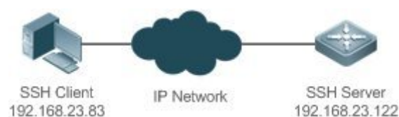
Figure 10-5 Networking Topology of SSH File Transfer
