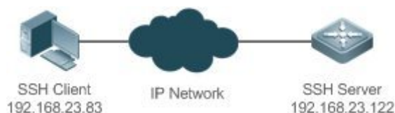
Figure 10-1 Networking Topology of SSH Device Management
