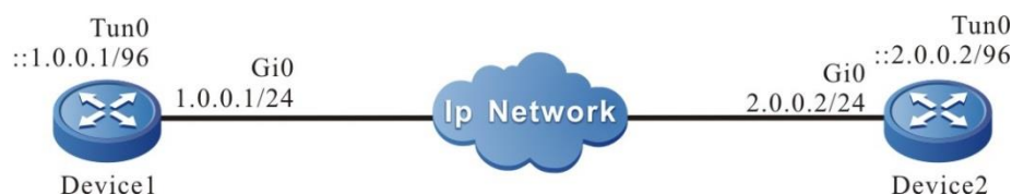
Figure 11-2 Networking of configuring the basic functions of IPv4 compatible IPv6 auto tunnel
