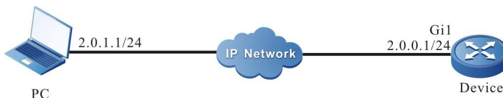
Figure 2-11 Configure the local device to log into the remote device via web
