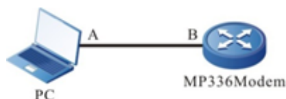
Figure 2-4 Description of connection method through remote dialing
