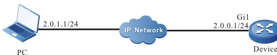
Figure 2-5 Network Topology for Configuring a Local Terminal to Telnet to the Device
