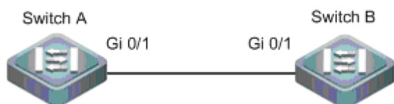
Fig 5 Basic topological diagram of LLDP
