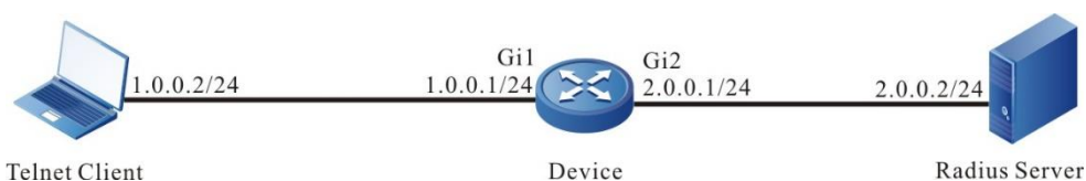
Figure 6-5 Networking of configuring Telnet user to carry different domain names to log in and use different authentication/authorization and accounting methods
