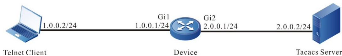
Figure 6–10 Networking of configuring the TACACS authorization and accounting of the Shell command
