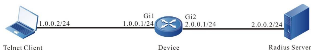
Figure 6-3 Networking of configuring Telnet user login to use RADIUS authentication/authorization and accounting
