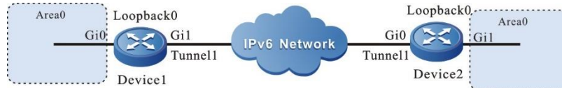
Figure 9-9 Networking of configuring IPsec tunnel to protect the packets of the GRE OVER IPv6 tunnel
