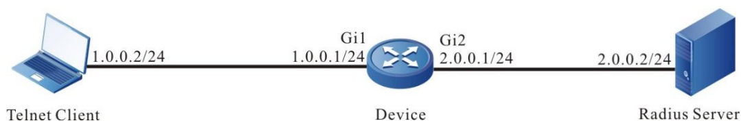
Figure 3-5 Networking of configuring Telnet user level switching to use RADIUS authentication
