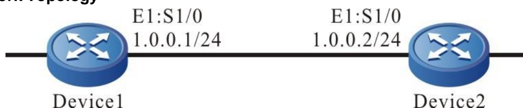
Figure 5-3 Networking of E1 framing CCS mode
