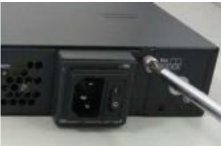
FIGURE 0-9 TIGHTENING THE FASTENING SCREWS
