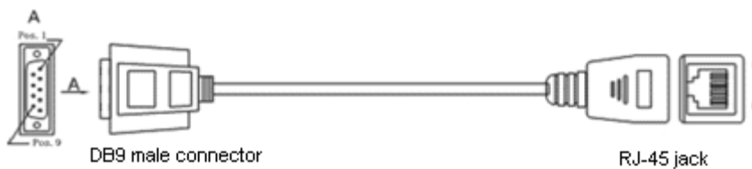
FIGURE 0-9 BALANCED CABLE WITH THE RJ-45 JACK
