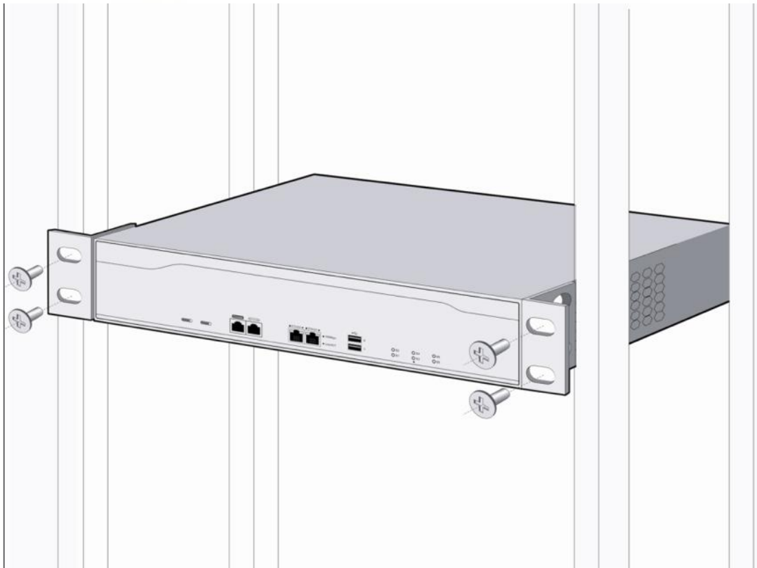
FIGURE 0-3 STEP 2-MOUNTING THE ROUTER ON A RACK
